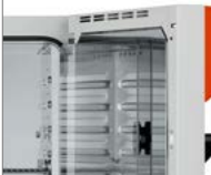
Inner door made of tempered safety glass
