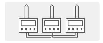
This is the standard method of control for all Carbolite Gero 3-zone furnaces. When the operator adjusts the setpoint of the centre zone controller, the setpoint of both end zones are automatically set to the same value. When a program is run in the centre zone all zones will automatically follow the program. Each controller has one thermocouple positioned with the tip close to the centre of each zone.
