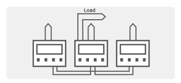
As in single zone furnaces, cascade control allows faster heating of the furnace load and more precise control of the load temperature. A CC-T1, EPC3008P10 or nanodac $^{\text{TM}}$  controller is required.
