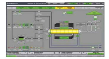
A touch panel interface is used for automated operation. All valves, temperatures, gas flows, etc. can be switched on and off manually or automatically by a predetermined program.
