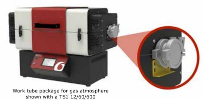
Detail showing the work tube support bracket. Work tube packages with extended length work tubes include guards and support brackets as indicated in this image.
