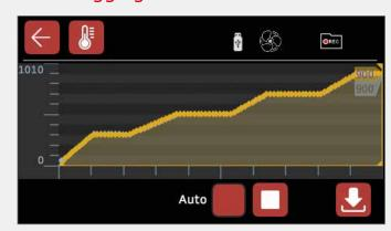
The data logging screen shows a graphical view of the setpoint and actual temperature along with the status of any configured relays. Data is logged to a USB stick in a .csv file format. Data logging can be started manually or automatically when a program is run.
