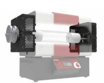
Work tube packages with extended length work tubes include guards as indicated in this image. The guards simply hook into the end plates of the tube furnaces and are each fixed with one screw.
