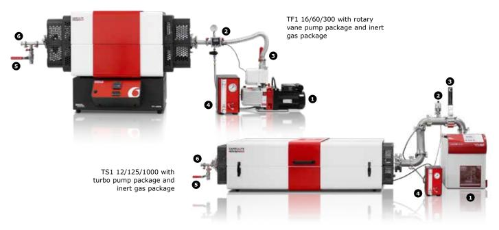
In a cold, clean, dry and empty furnace the rotary vane pump option is able to reach a vacuum level of 5 x  $10^{-2}$  mbar, the turbo pump option reaches under the same conditions  $1 \times 10^{-5}$  mbars.
