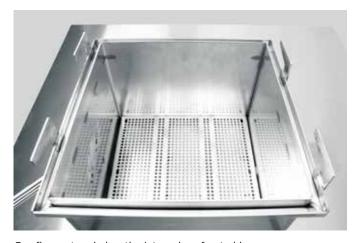
Gas flow enters below the internal perforated base  $% \frac{1}{2}\left( \frac{1}{2}\right) =\frac{1}{2}\left( \frac{1}{2}\right)$
