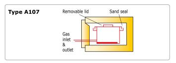
The A107 NiCr alloy (Inconel) retort with a shallow removable lid locates into a sand seal on top of a deep base. Can be used for annealing and pack carburising. Front mounted gas inlet/outlet connections extend through slots in the furnace door.
