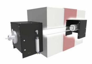
Attachment housings can be secured to the furnace for convenient vacuum / protective gas operation.
