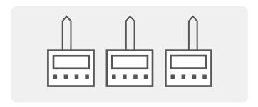
This configuration comprises independent controllers, each with an independent thermocouple in its respective zone. This is the standard method for the TG gradient tube furnaces.
