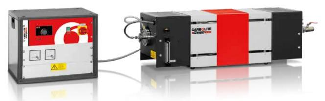
${\it FHA~13/80/500~with~optional~CC-T1~controller,~voltage/current~display~and~high~vacuum~capable~inert~gas~package.}$ Rotary vane pumps and turbo pumps available (see page 112)
