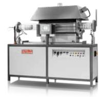
Bespoke cycling corrosion test furnace
