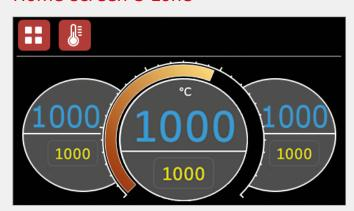
For a 3-zone product the home screen shows the setpoint and actual temperature of each zone. The user can select the end zones to either follow the centre zone temperature or run independently.
