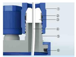
Schematic diagram of GLS 80® connection system
