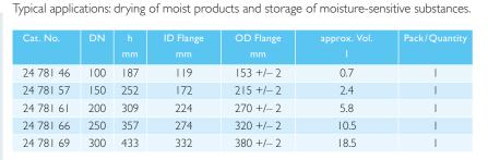
Desiccator lid made from DURAN® borosilicate glass 3.3. Components are vacuum tight
