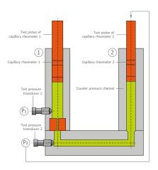
The RG Counter Pressure offers the opportunity to automatically measure different viscosity functions under counter pressure. Capillary rheometer 2 regulates counter pressure. After a flow curve is determined, the material is being pushed from capillary rheometer 2 into capillary rheometer 1. Now, a flow curve can be measured under different counter pressure. The illustration shows a schematic example of two connected capillary rheometers.
