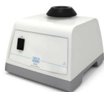
RX3 Electronic speed regulation: Constant 3000 rpm
