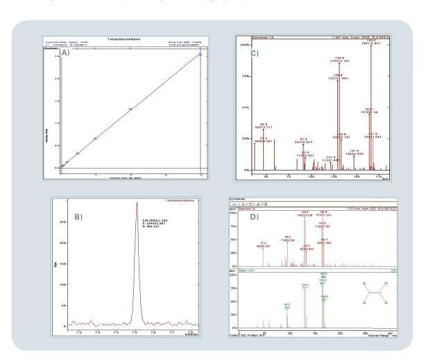
(A) Excellent linearity of Tetrachloroethylene from 0.1 to 40 ppb with the purge-and-trap, (B) good sensitivity, (C) high quality spectra, (D) down to 0.1 ppb level and showing good match to the NIST library.
