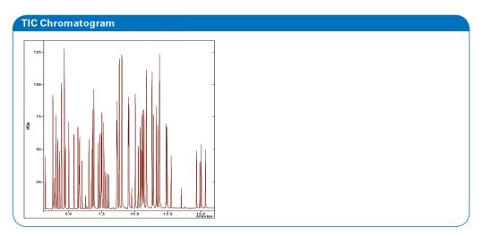
TIC chromatogram of a 5 mL water sample containing 84 VOCs at 10 µg/L (ppb) by US EPA Method 524.3
