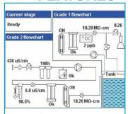
System flowchart shows all component status and water quality parameters at a glance.
