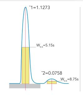
The graphic shows the absorbance peak for a 1-mg/kg mercury solution and the subsequent profile of blank run.
