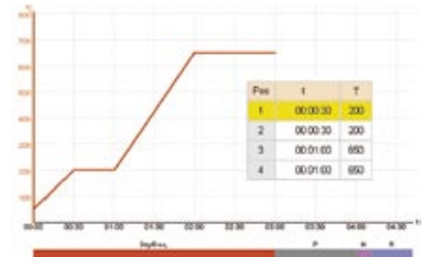
Typical drying/decomposition temperature profile for Naphtha samples.
