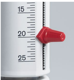
Positive volume setting using interior scalloped track
