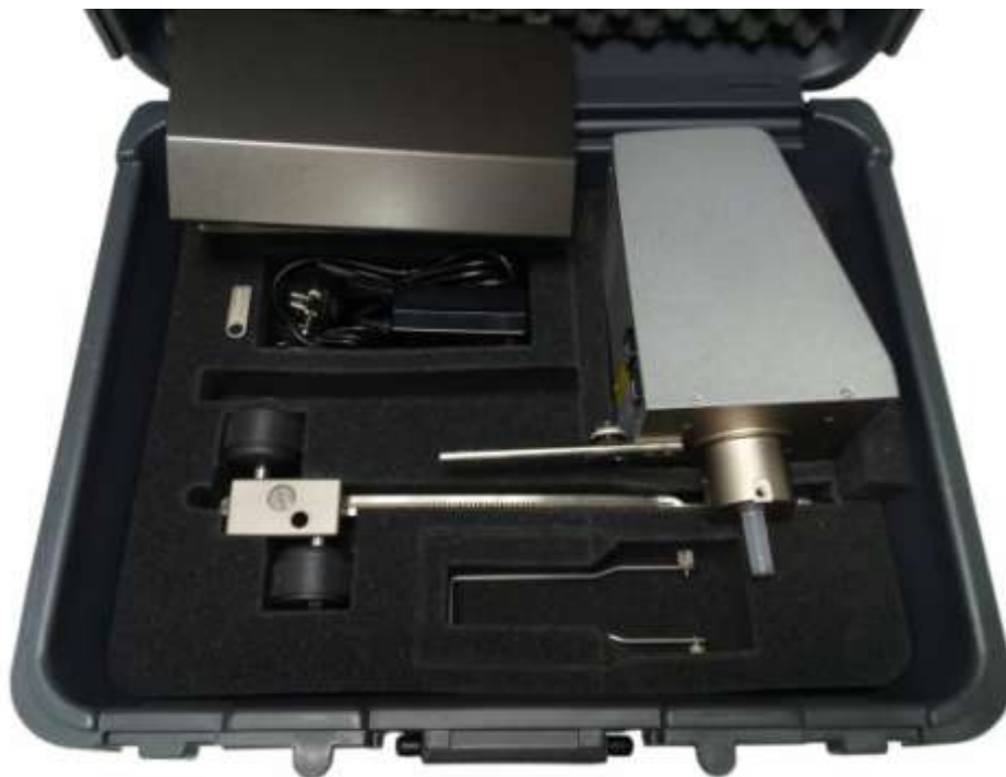
Fig. 1.b Second level of the viscometer in its carry-case
