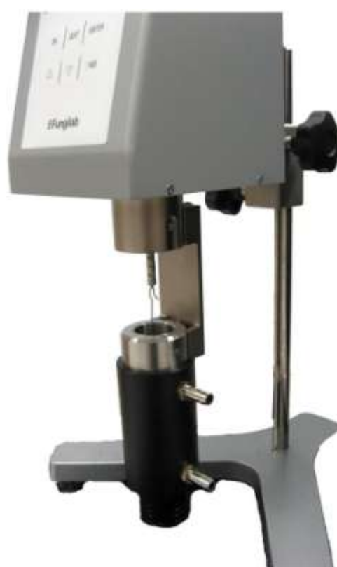
Fig.9: LCP Adapter assembled in viscometer
