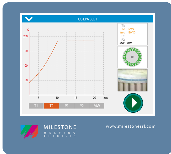
Temperature profile of a soil digestion in accordance with US EPA 3051 using the MAXI-44 rotor
