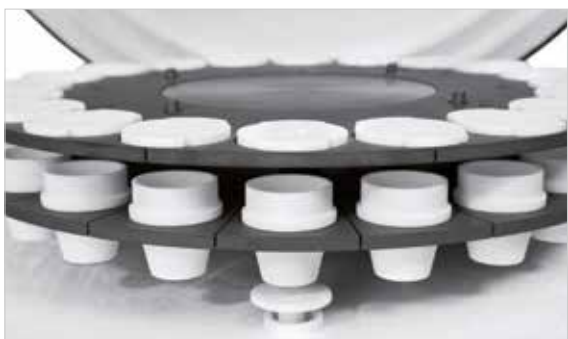
PC-controlled application of crucible lids / crucibles open
